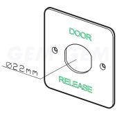
Switch Ratings : 5A@125 Vac Type of Actuation: Momentary Contact Arrangement: Double pole double throw Operating travel: 2.7mm Operating temp. Range: -20~+70C Contact resistance: 50mÜ Max.(initial) Operating life(Mechanical): Over 100,000 times Materials: Zinc alloy
